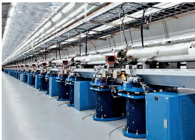
The 132 m long undulator is part of the world's currently most powerful X-ray laser at the SLAC National Accelerator Laboratory in California.
